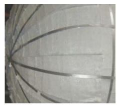
**Pyrogel XTF** incorporates all the insulative qualities of Pyrogel XTE to combine classleading thermal performance with versatile passive fire protection. Hydrophobic and breathable, Pyrogel XTF keeps underlying assets drier for longer, providing superior corrosion defense and maintaining process conditions in the harshest of environments.
