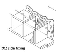
Besides the MAS modules we are able to supply you with other types of modules (for example folded and bonded) and various types of anchoring systems. The anchor lock modules can be supplied with either side fixing (RX2) or central fixing (thread lock and weld lock) anchors.
